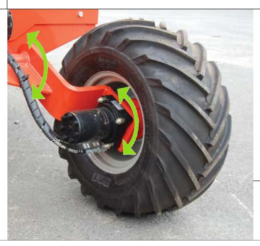
The front traction wheels are hydraulically powered and independant in their movements, providing a total even traction in any given situation.
