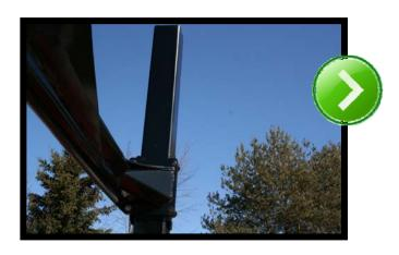
The fork is built to minimize contact with the net wrap.
