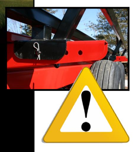
Rails exceed the length of the deck to secure the bales on the back portion of the trailer assuring stability in transport.
